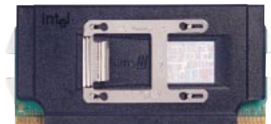
Example of an incorrectly installed retention clip
