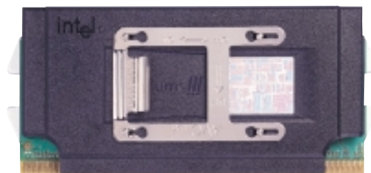
Example of an incorrectly installed retention clip
