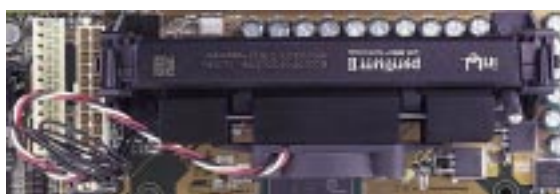
Pentium II processor packaged in an SECC with heatsink and fan (top view)
